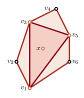
Fig. 2.4: x can be written as a convex combination of  $v_1$ ,  $v_3$  and  $v_5$ .
