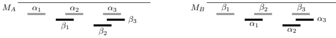
Fig. 1. Instance where A^3 returns exactly 2/3 \cdot |O| jobs: O contains all jobs \alpha_i and \beta_i for i = 1, 2, 3 (in grey), but both A^2(M_A, M_B) and A^2(M_B, M_A) schedule only the jobs \alpha_1, \alpha_2, \beta_1, \beta_2 .
