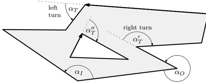
Figure 4: A polygon with one hole. Marked inner angle  $\alpha_I$ , outer angle  $\alpha_O$  and three turn angles  $\alpha_T > 0$ ,  $\alpha'_T < 0$ , and  $\alpha''_T < 0$ . Observe that  $\alpha_T$  and  $\alpha'_T$  are the turn angles in counterclockwise direction, whereas  $\alpha''_T$  is the turn angle in clockwise direction.
